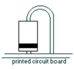
Resistors R5, R6, R7, R8, R9 & R10 also mount vertically. We suggest that the position of R7 be reversed as shown in red on the right below. This will insure that none of the leads can touch those of other resistors.
