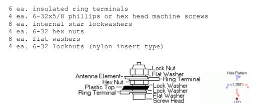
Remove the top cover from the enclosure. Drill 4 holes in it for the 6-32 screws. The holes are in a symmetrical diamond pattern with about 1-1/4 inches cross corner. The elements can also be mounted atop the MR26A or MR26E.
