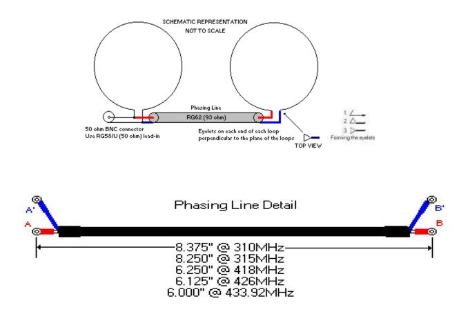
For clarity, the schematic representation above shows the loops separated but they are assembled perpendicular to each other with one loop inside the other as shown on the following page.
