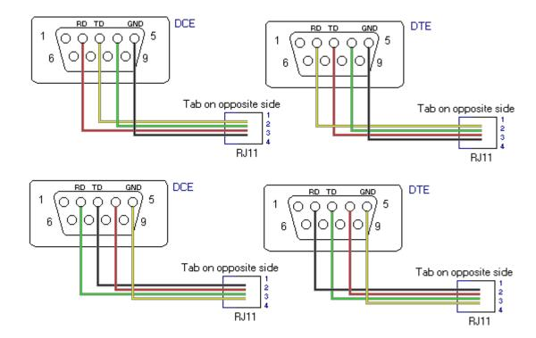
The DCE cables shown above work for the Ocelot and all DCE devices that use a DB-9 connectors. A DTE cable or a null adapter is required to connect one of the Gateway's secondary ports to a PC serial port for Irman emulation.
